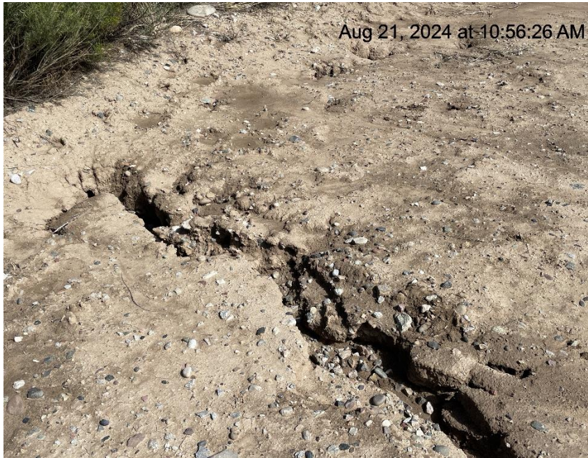
Photo # 5594 Tunnel erosion & transport of sediment off location
