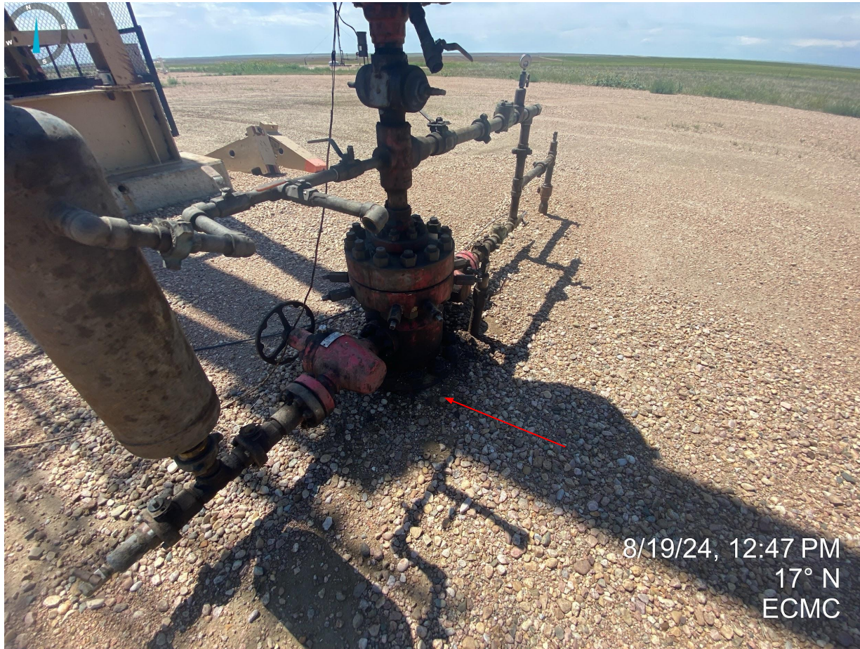
Photo 11. Stained soil around wellhead.
