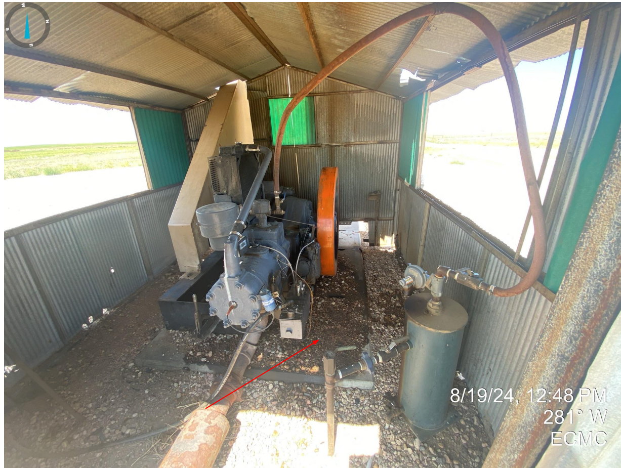
Photo 13. Hydrocarbon staining at pumpjack motor.
