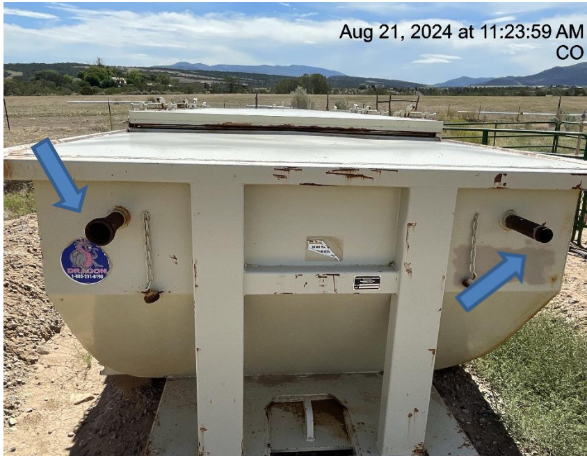
Photo # 5709 Open ended piping/wildlife hazards on unused equipment
