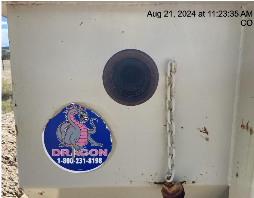
Photo # 5711 Open ended piping/wildlife hazard on unused equipment
