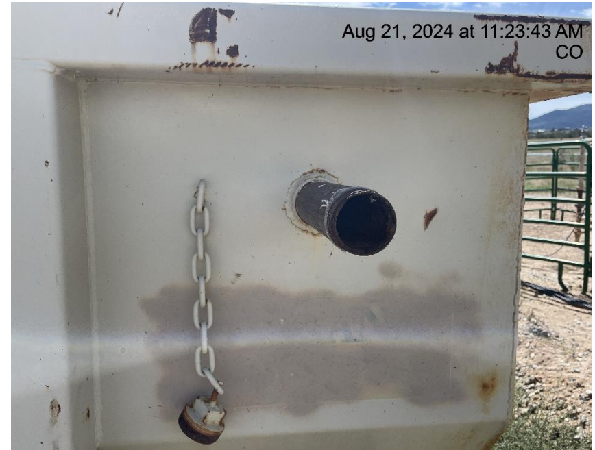
Photo # 5710 Open ended piping/wildlife hazard on unused equipment
