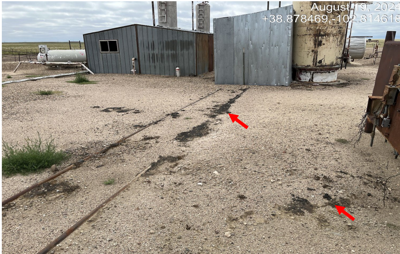
Photo 7. There are oil stained soils along the flowlines that go to the heater treater.
