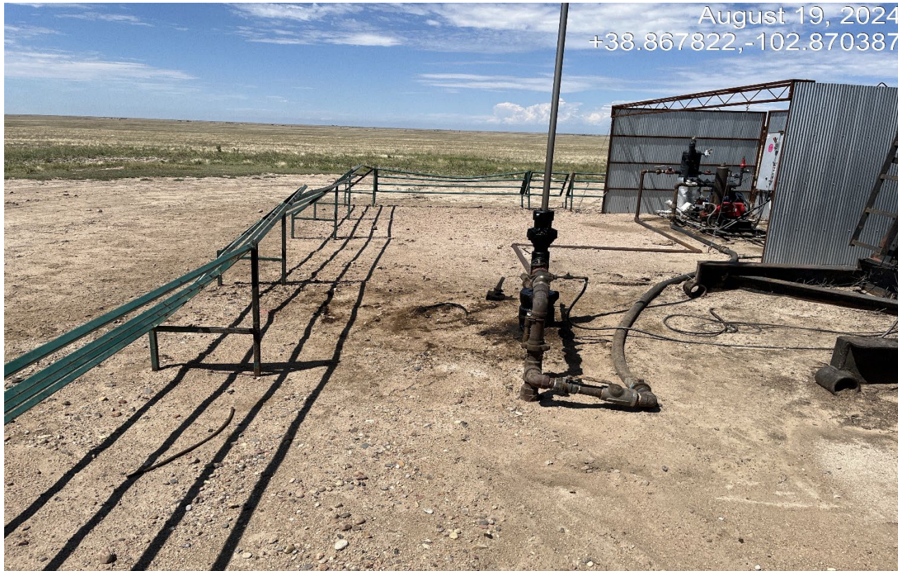
Photo 4. There is oil stained soils at the wellhead that needs to be cleaned up..
