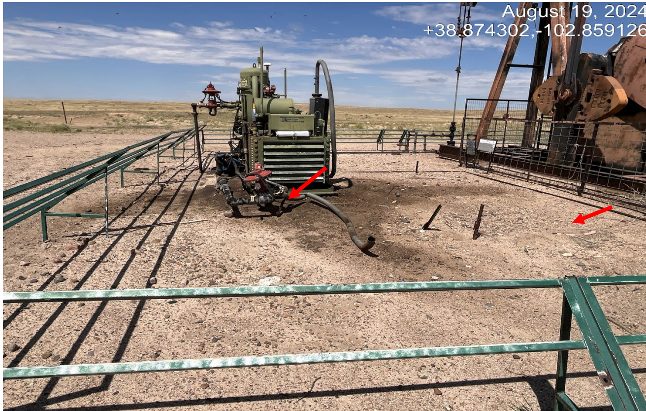
Photo 4. There is stained soils around the engine that needs to be cleaned up. There is a bucket of oil not properly stored with containment. There is a metal panel laying on the ground next to the shed.
