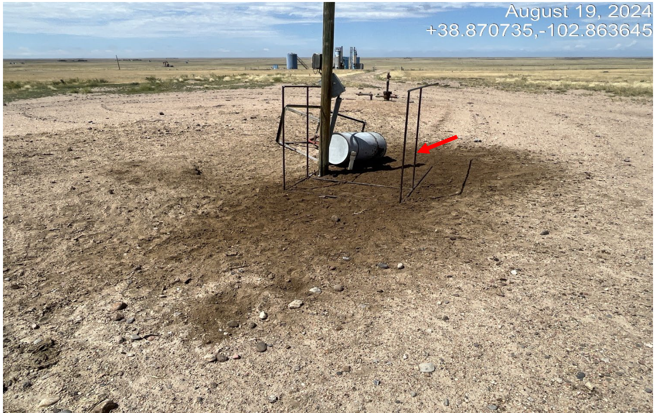
Photo 3. There is dark oily soils and a tipped over chemical drum. Stained soils must be cleaned up and unused equipment removed.
