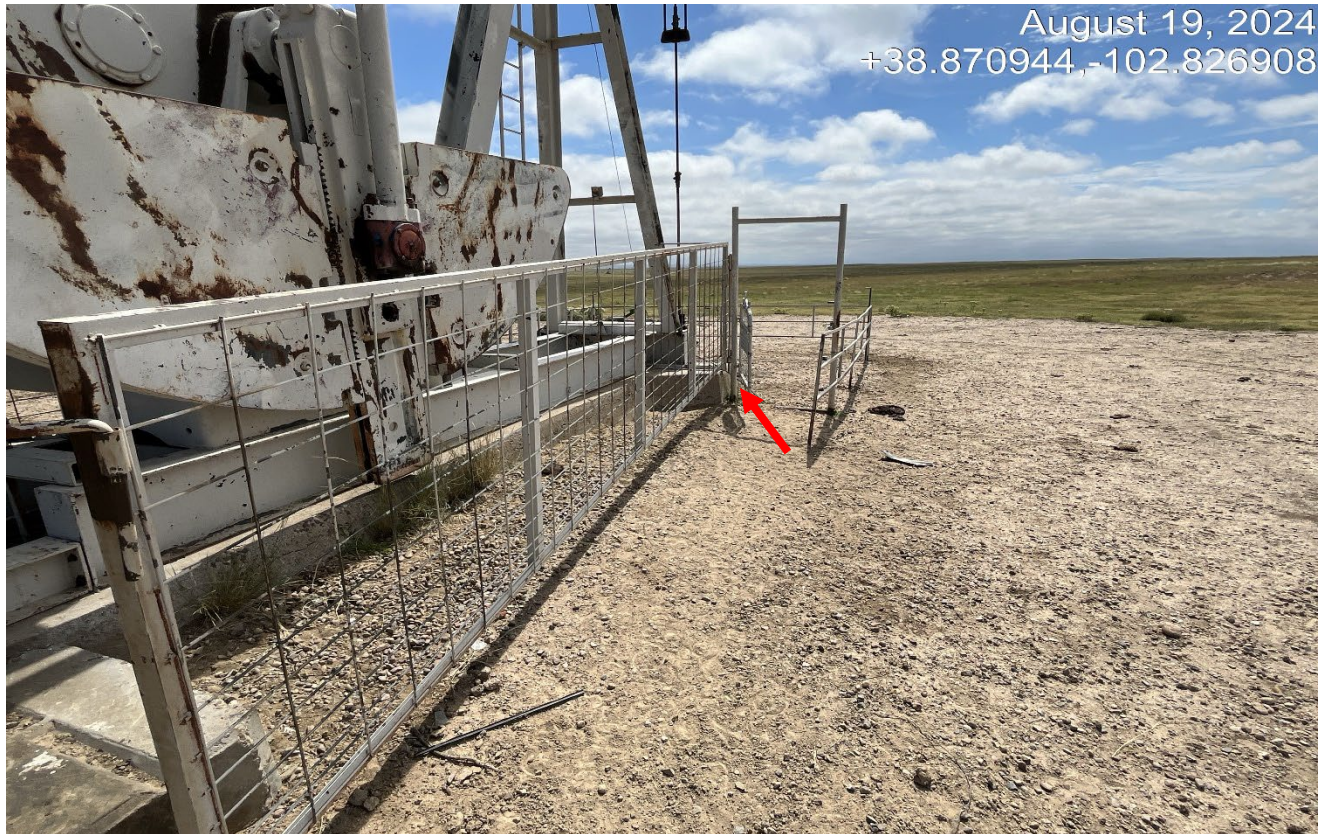
Photo 2. Facing at the pumpjack. The gate was left open and livestock entered in the enclosure. The well sign on the gate is obstructed from view.
