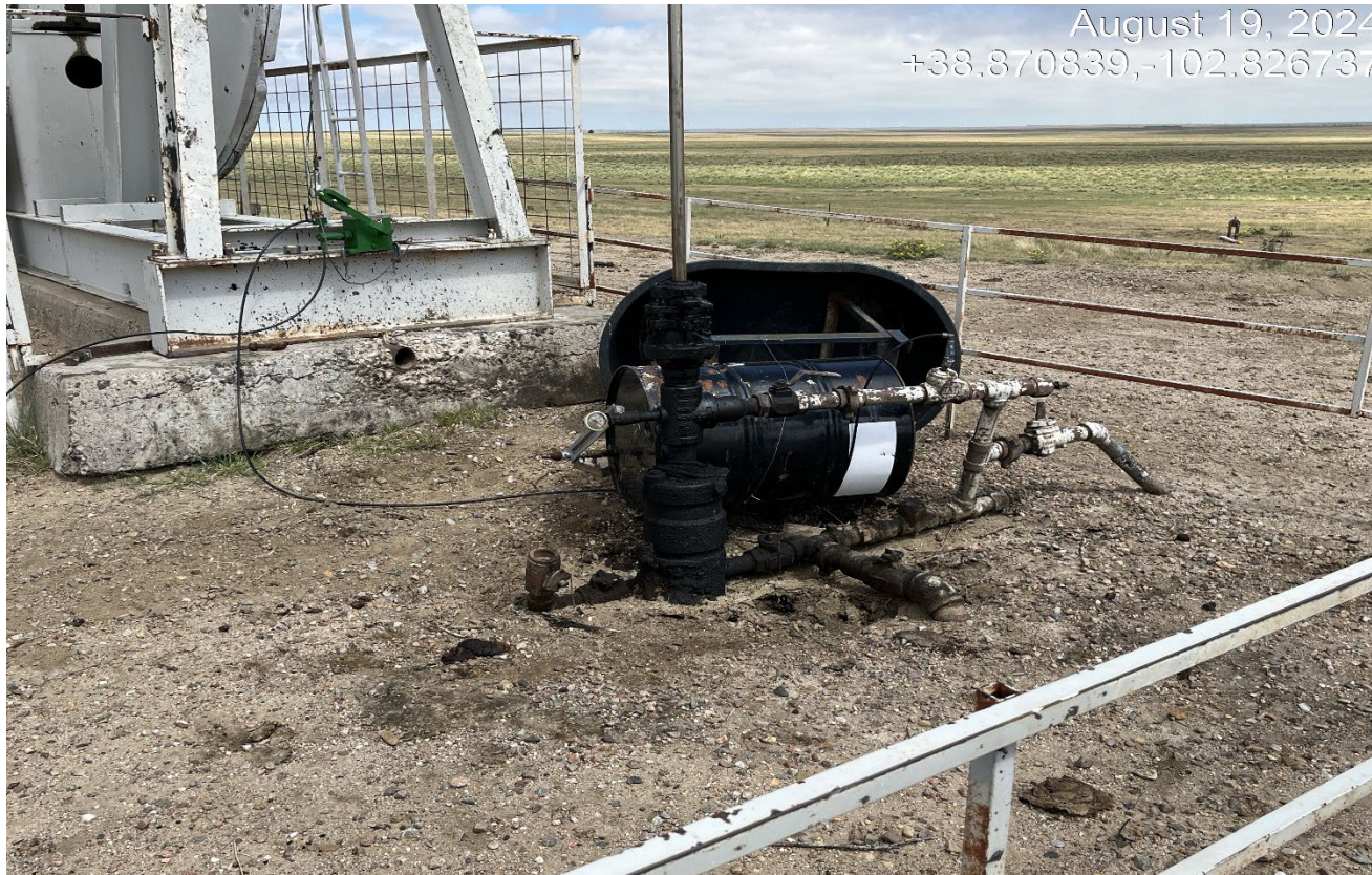
Photo 3. The chemical barrel has tipped over and there are signs that livestock was inside this enclosure. There is oil stained soils at the wellhead.
