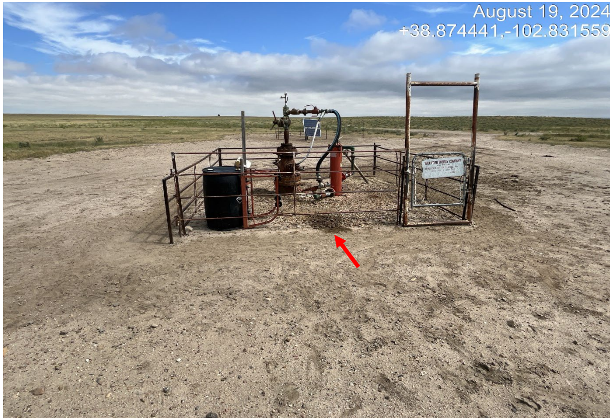
Photo 3. The well sign is faded and not legible. There is oil stained soils at red arrow. There is a chemical barrel with no secondary containment..
