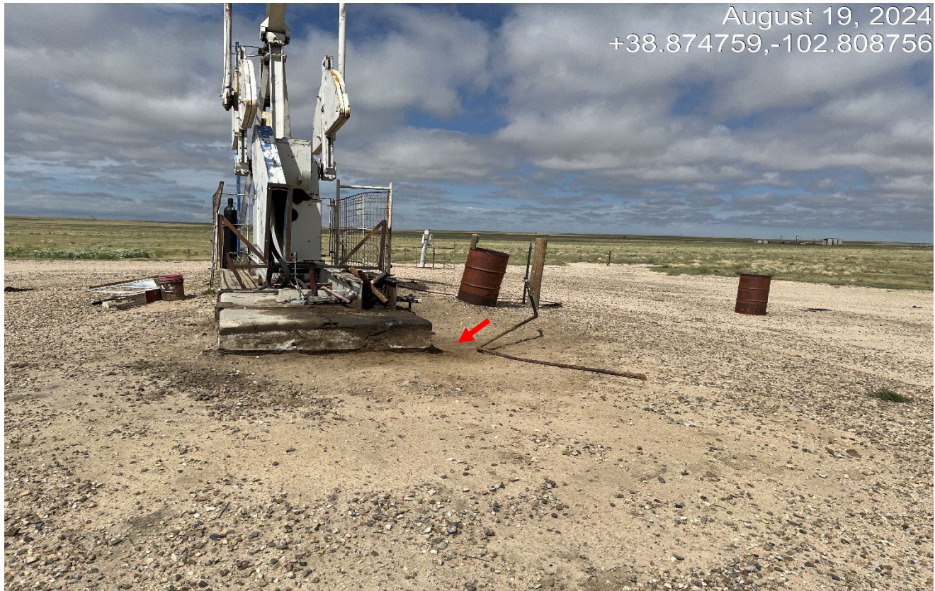
Photo 6 . Facing northwest at the pumpjack. There are stained soils at red arrow and parts laying on the ground.
