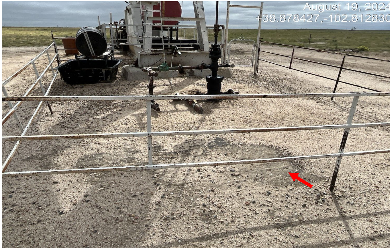
Photo 10. Facing toward the wellhead. There are stained soils by the wellhead shown at red arrow.
