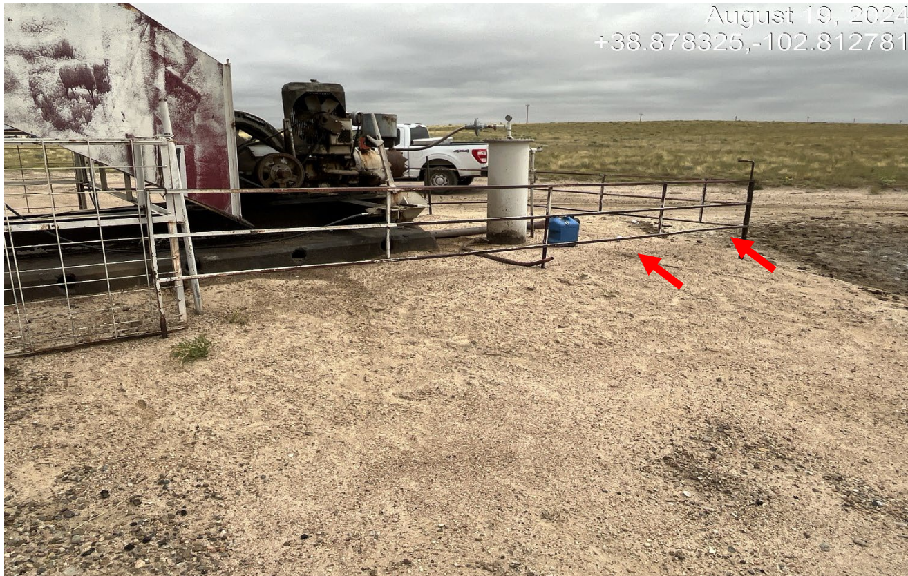
Photo 4. Facing toward the pumpjack engine. There was new sand spread around the pumpjack base to cover up the stained soils which were not cleaned up. There are three cans of starting fluid and the blue can that need to be removed.
