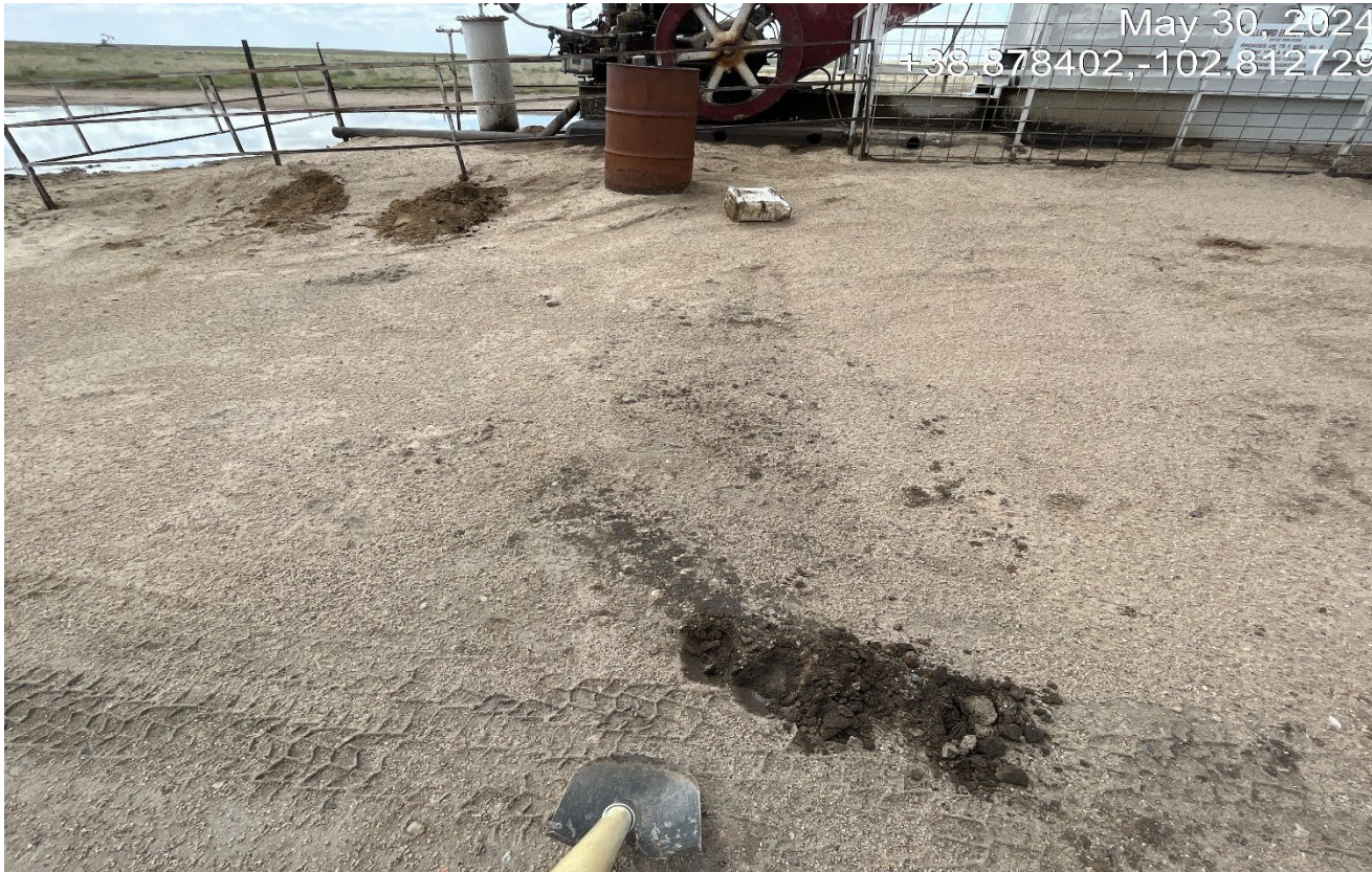
Photo 8. There is impacted soils about 15 ft. north of the pumpjack engine.
