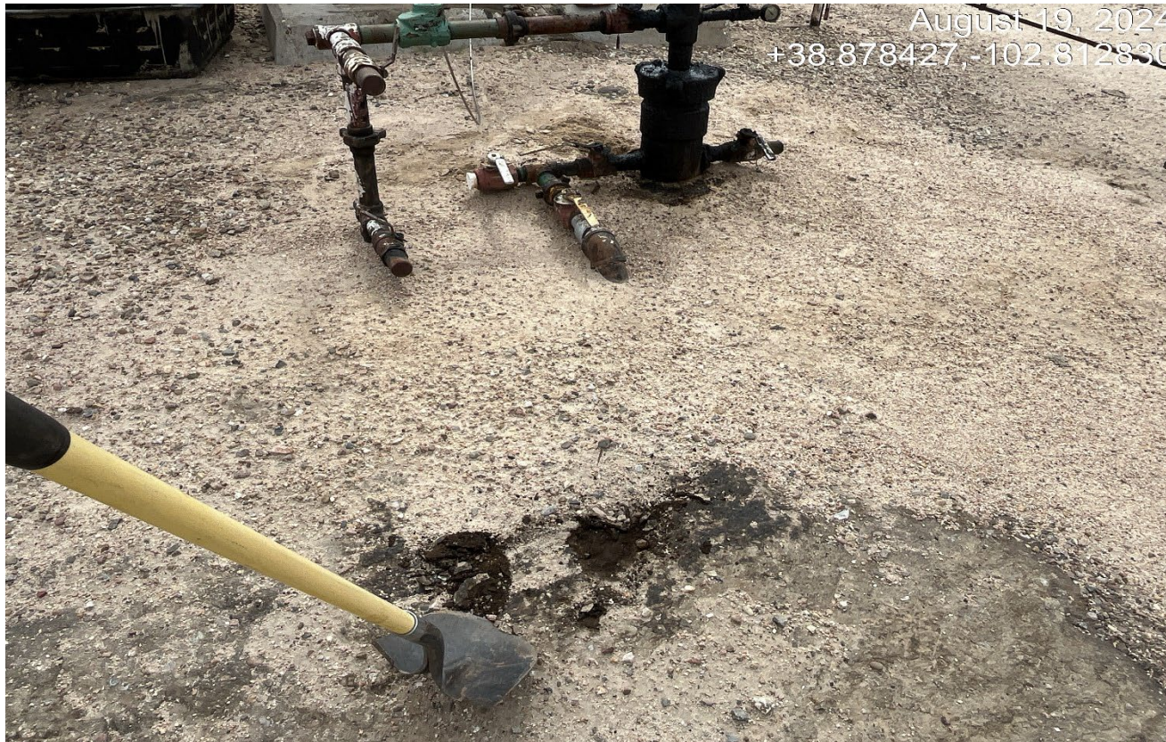
Photo 11. Scratching the soils by the wellhead show oily saturated black staining from E&P waste.
