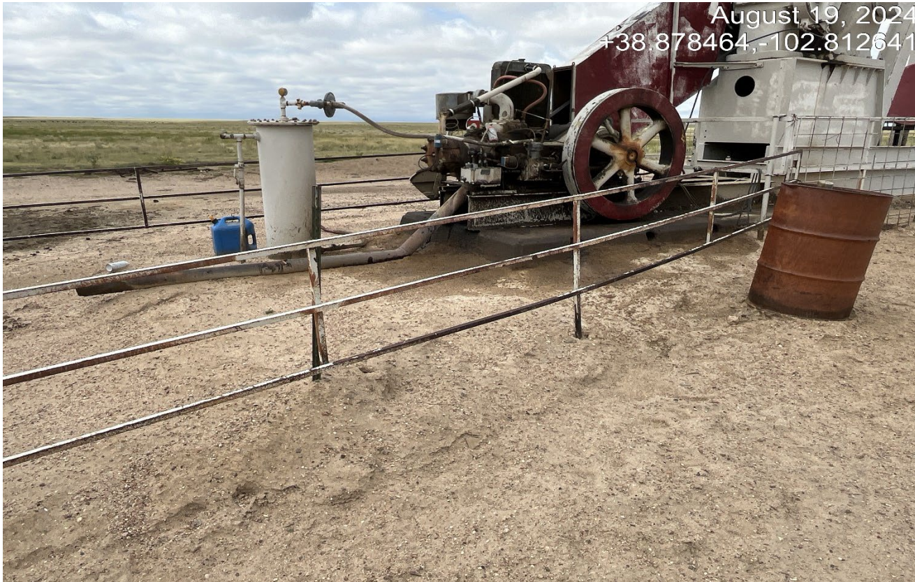
Photo 6. The pumpjack engine is still leaking oil.
