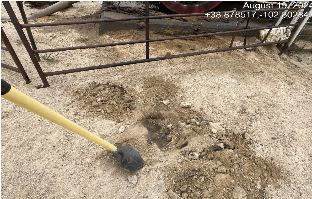
Photo 6. It appears there was sand spread on top of the spill which was not cleaned up per the rules. There is still oily soils that remain underneath the sand that was placed over the stained soils.
