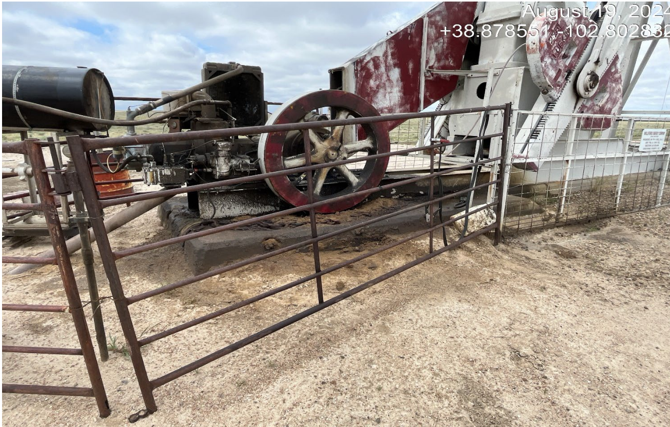
Photo 5. The pumpjack engine is still leaking oil and there is stained soils around the base.
