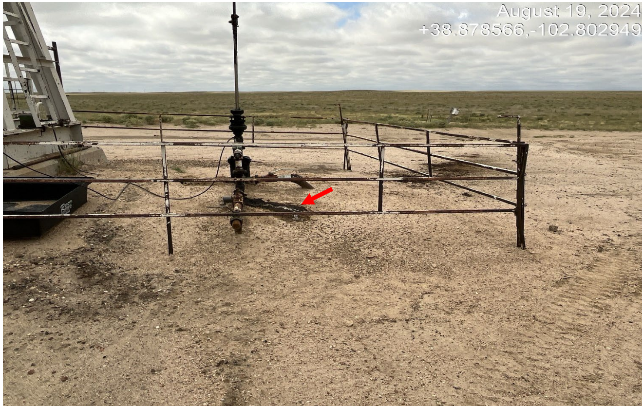
Photo 4. It appears there was sand spread on top of the spill which was not cleaned up per the rules. There is a new leak at the wellhead shown at red arrow.
