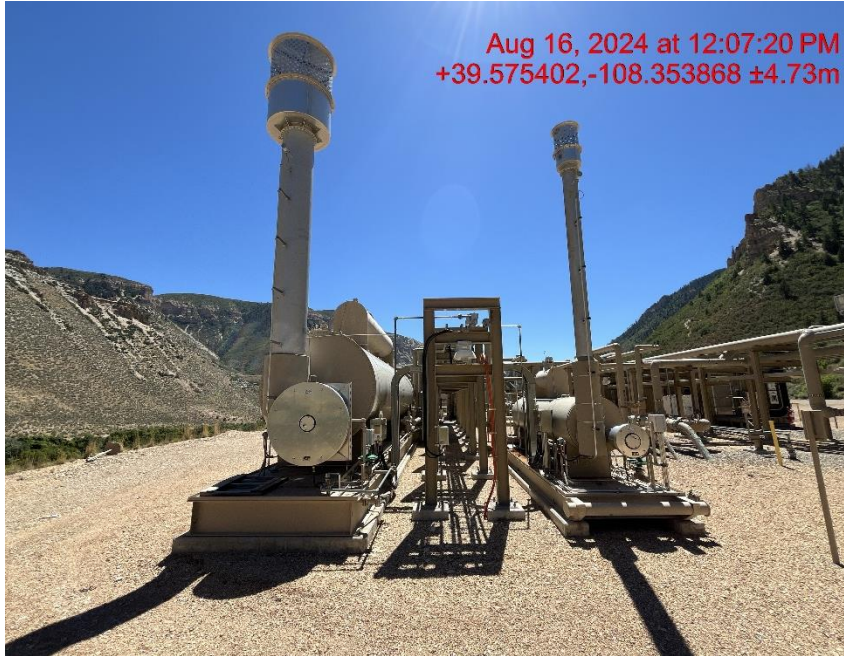
Line heaters/out of service - Photo #04725
