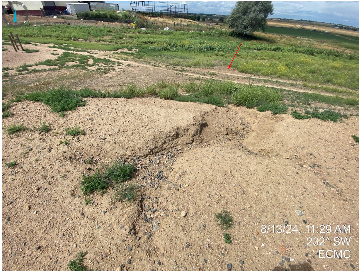
Photo 6. Continued from Photo 5; facing southwest. Photo illustrates erosion degradation (e.g. gullying) and sediment deposition off location (indicated by red arrow).
