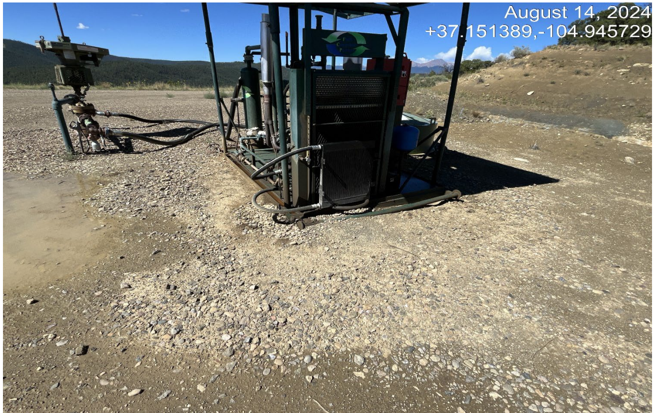
Photo 2. There is still oily fluid in the engine skid. It appears fresh base was placed where staining occurred. Stained soils should be removed and disposed.
