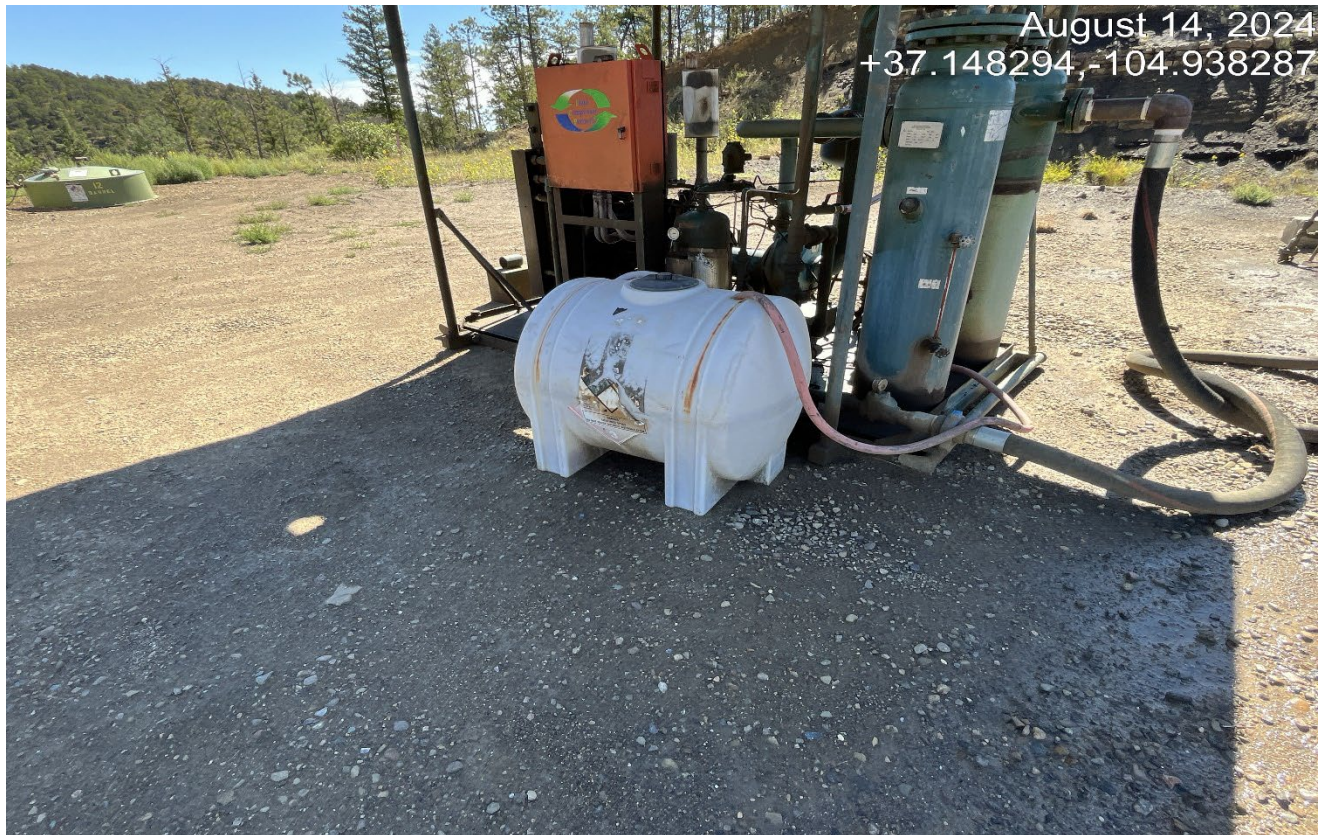
Photo 3. The labeling on this tank is degraded and needs to be replaced. This tank should also have secondary containment..
