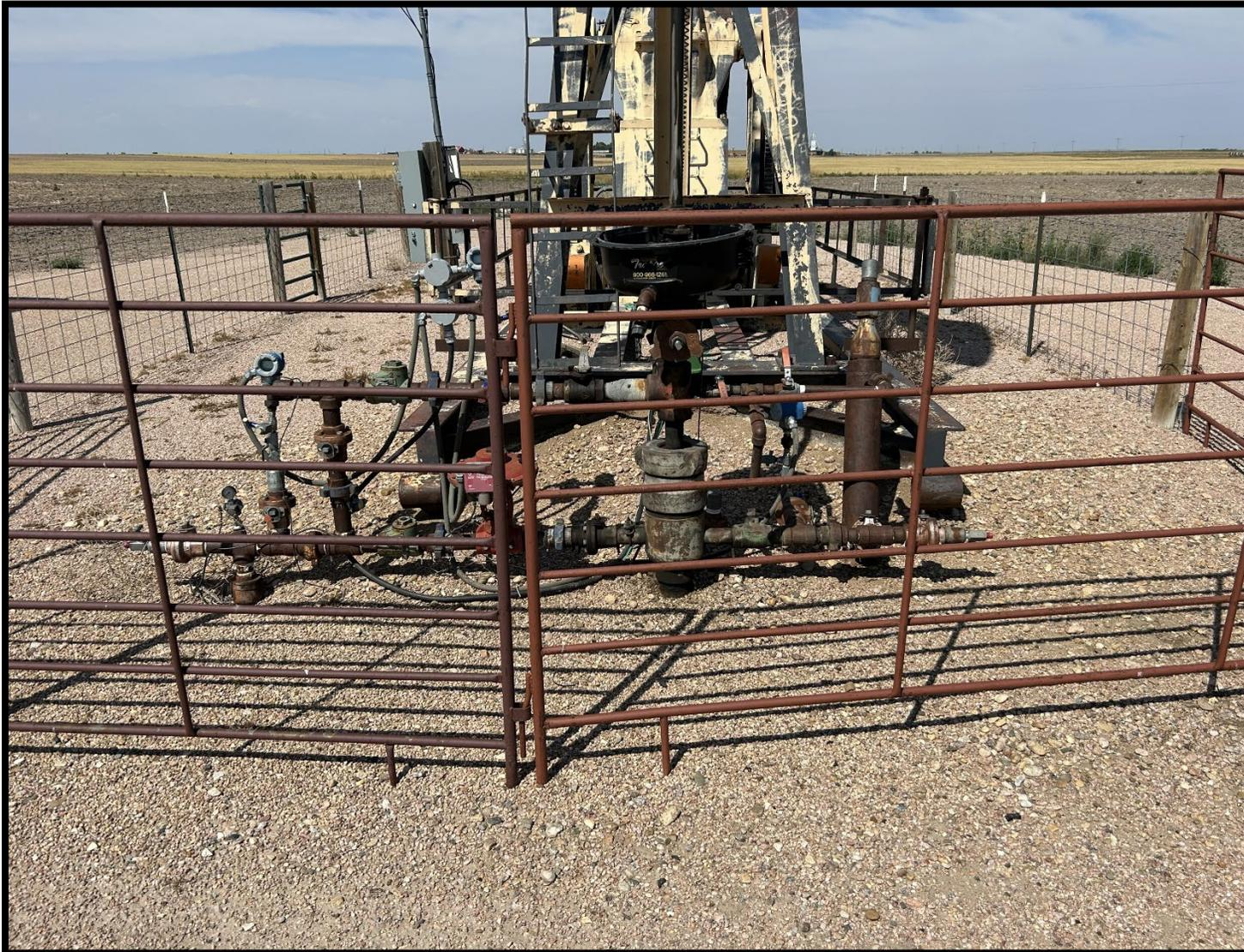
**CA:** Stained Soil at Wellhead. Properly treat or dispose of oily waste in accordance with 907.e.
