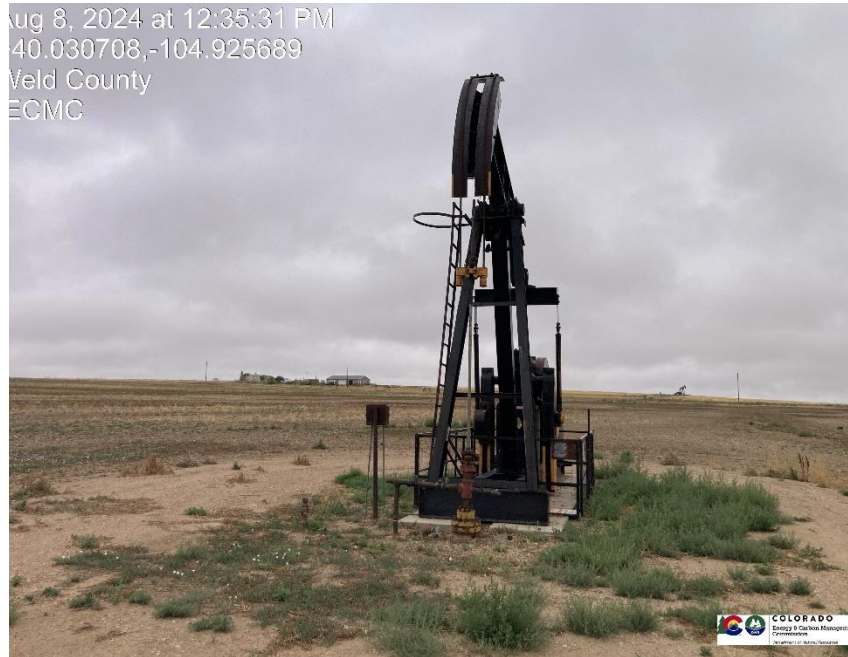
Pic 1 wellhead sign missing on wellhead / pumpjack
