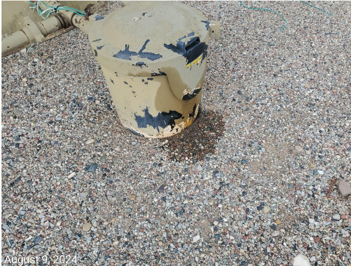
Photo 4: Stained soils at loadline.
