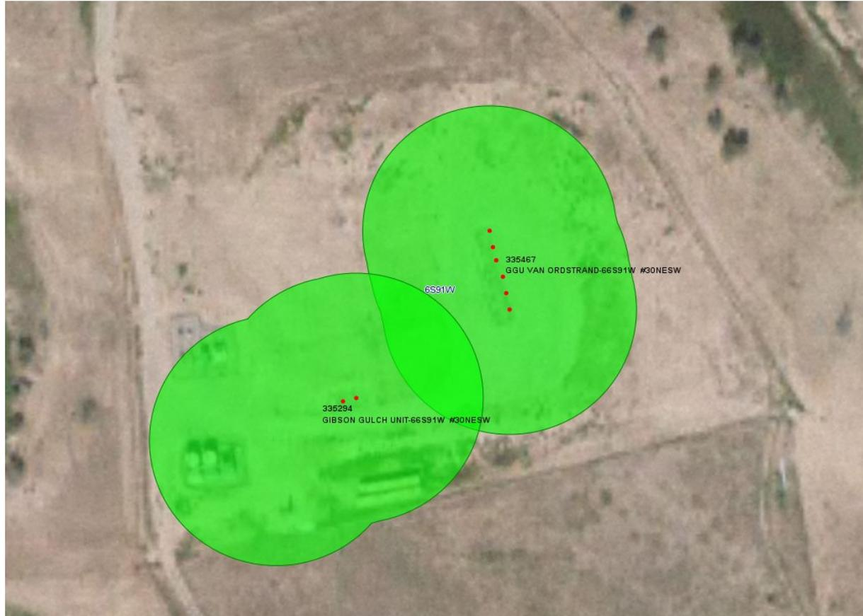
**Photo 5:** ECMC COGIS imagery. Photo shows flowline systems registered in the area; no Off-location flowlines have been registered at the VAN ORDSTRAND Location; no other facilities exist on the Location; flowlines from the wells likely travel off-location to the tank facility on the GIBSON GULCH UNIT-66S91W/30NESW (#335294), to the west of the Van Ordstrand Location (#335467).
