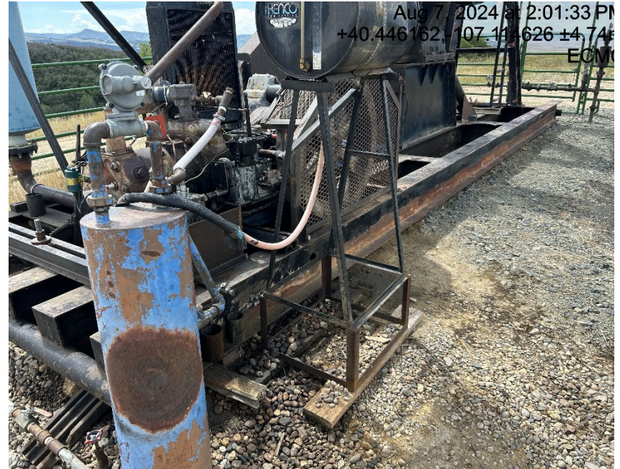
Unknown contents / no secondary containment / staining
