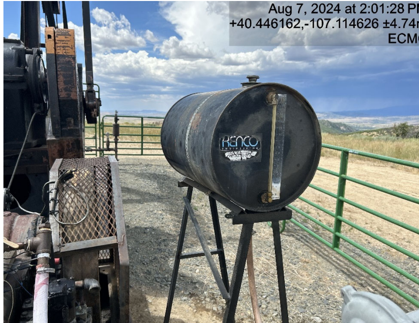
Unknown contents / no secondary containment
