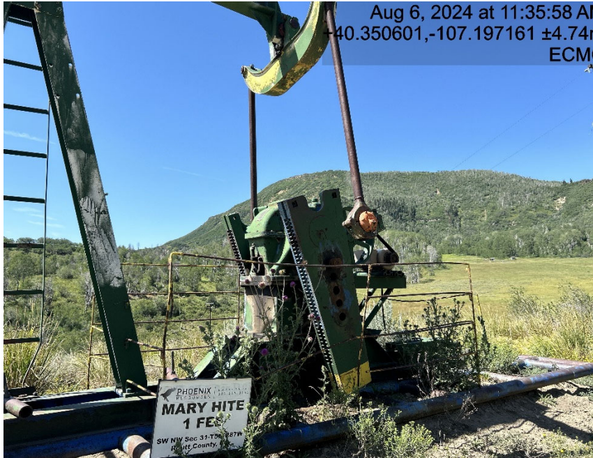
Well signage lacking information / weeds / broken equipment
