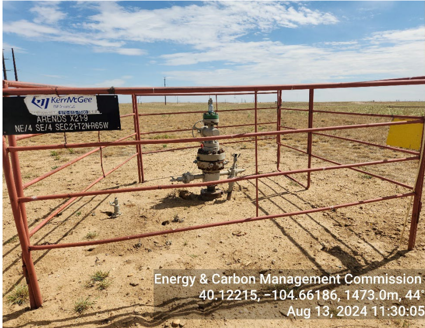
Photo 9: TA wellhead
