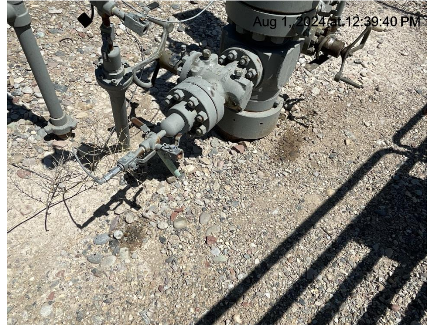
Photo # 4436 Staining near wellhead
