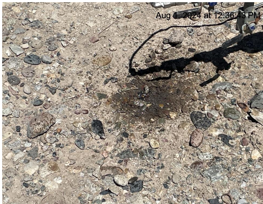
Photo # 4437 Staining near wellhead
