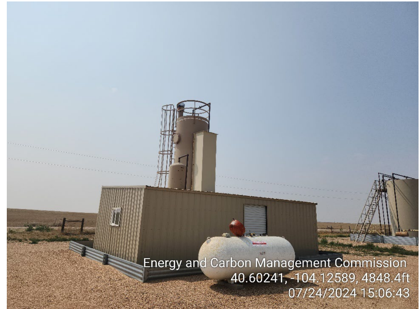
Photo 4 – Heater Treater
