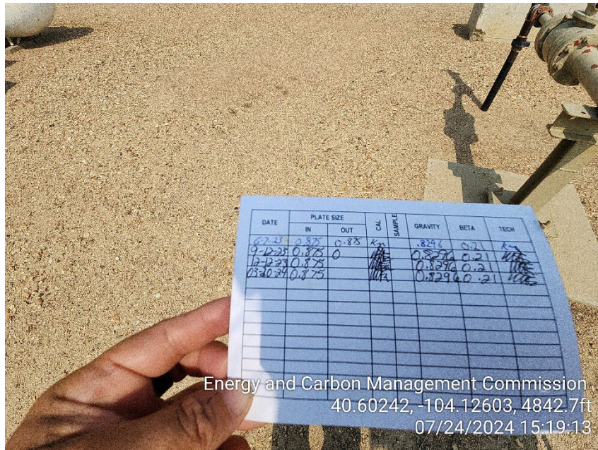
Photo 19 – Gas Sales Meter Calibration Card
