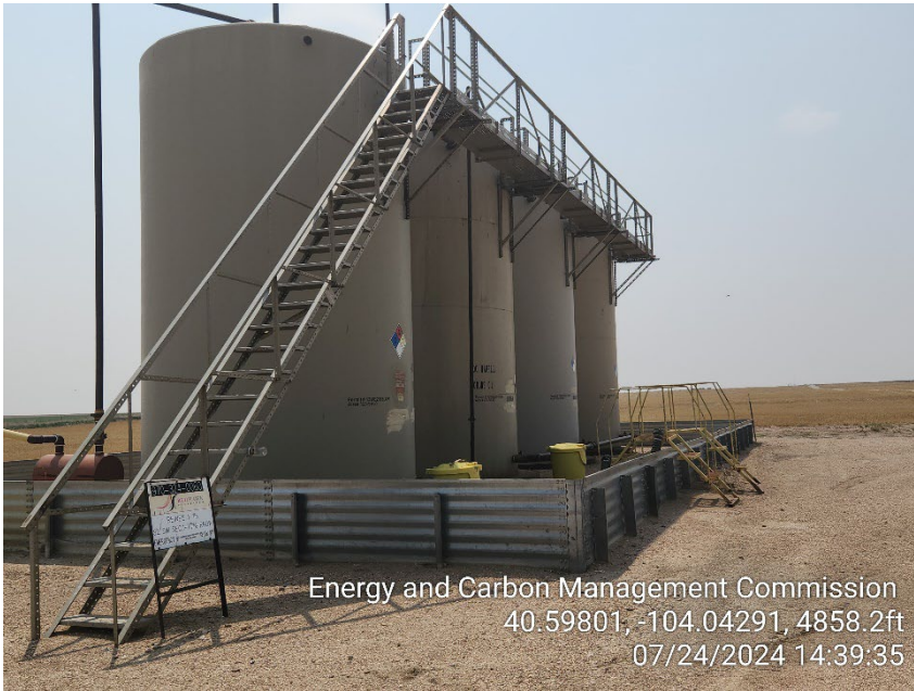
Photo 7 – Tank Battery
