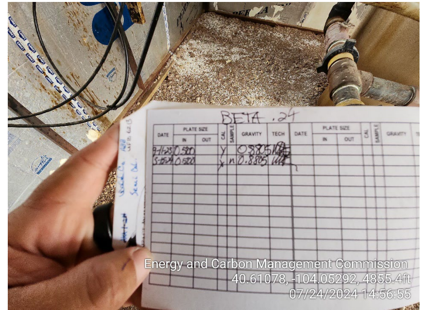
Photo 12 – Sales Gas Meter Calibration Card
