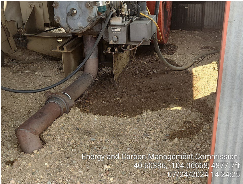
Photo 3 – Stained Soil at Gas Engine
