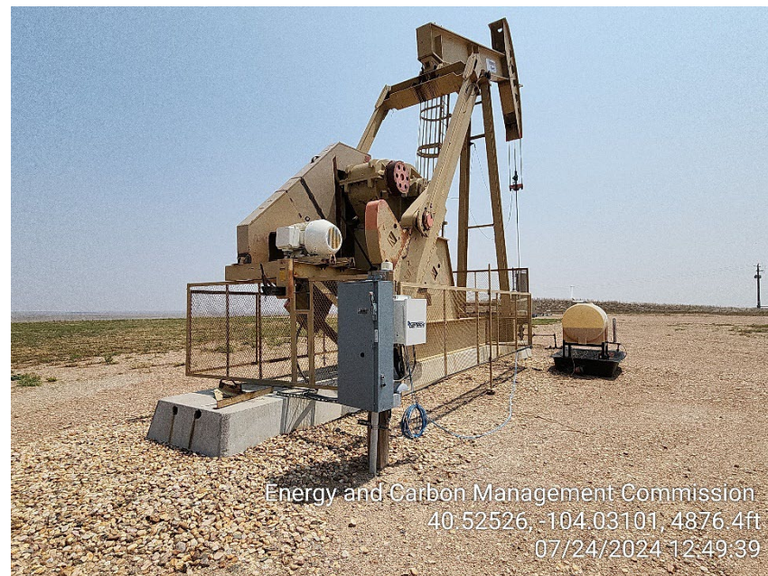
Photo 4 – Electric Motor
