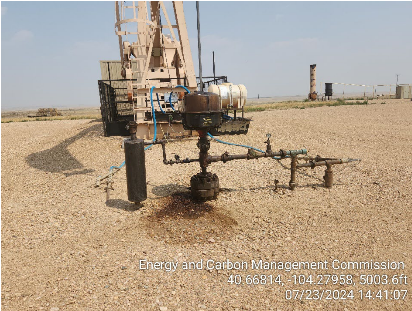
Photo 3 – Wellhead – Stained Soil
