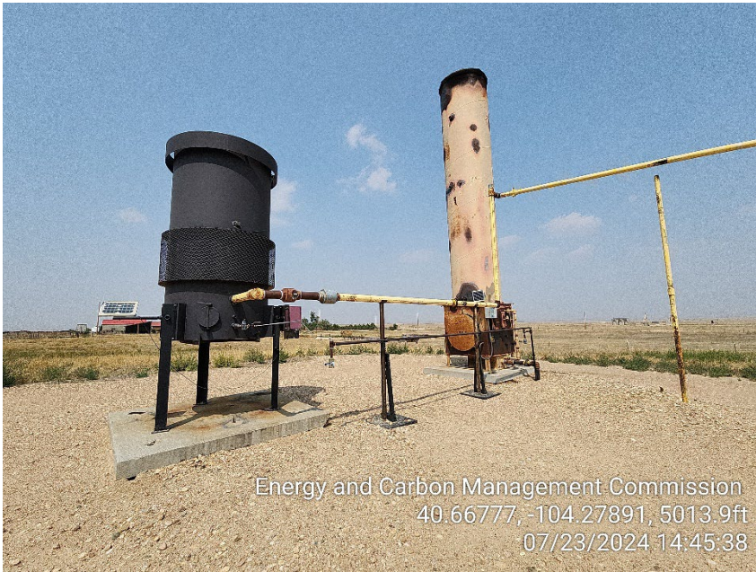
Photo 11 – ECD and Combustor
