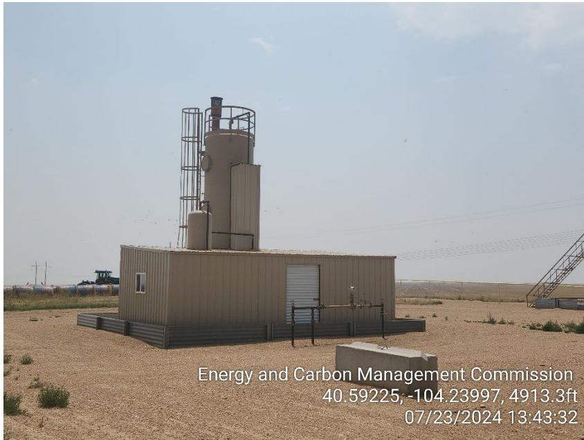
Photo 3 – Heater Treater
