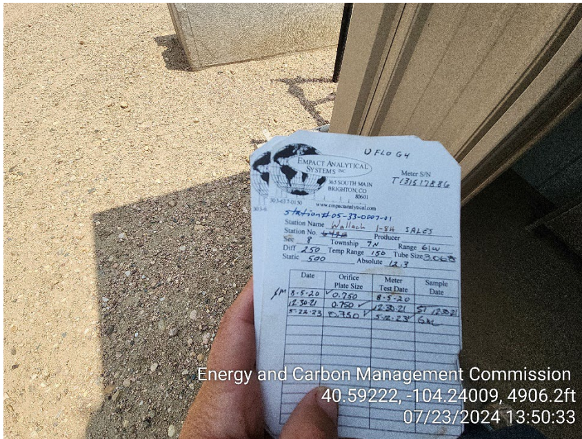
Photo 19 – Sales Meter Calibration Card
