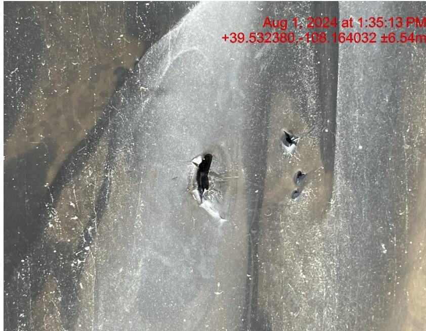
Holes in containment liner - Photo #03935
