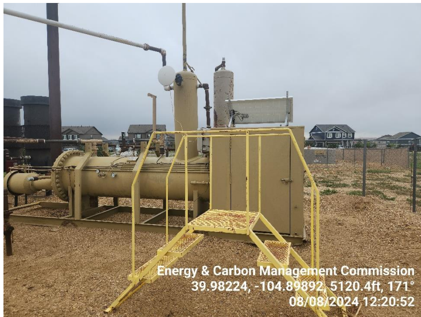
Photo 13 Horizontal Heated Separator.
