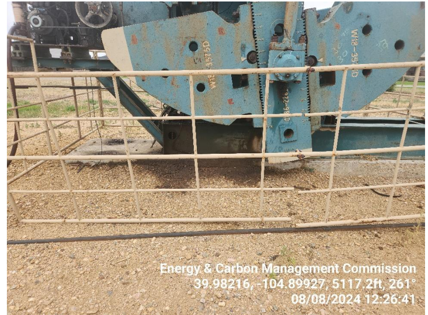
Photo 26 Stained soil on & at the Pump Jack base.
