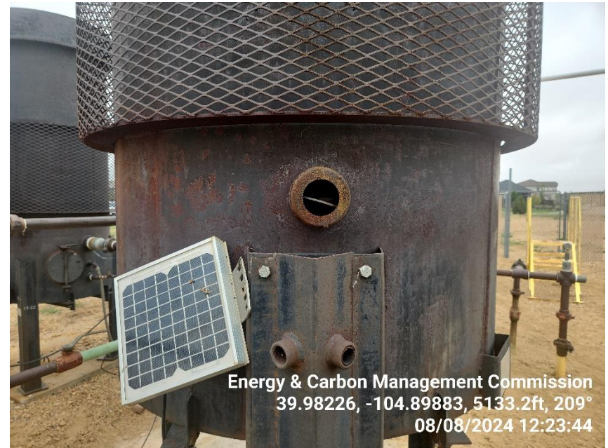
Photo 20 Damaged ECD sight glass.
