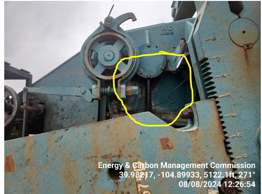
Photo 28 Pump Jack seal leaking oil onto the PJ base & ground.
