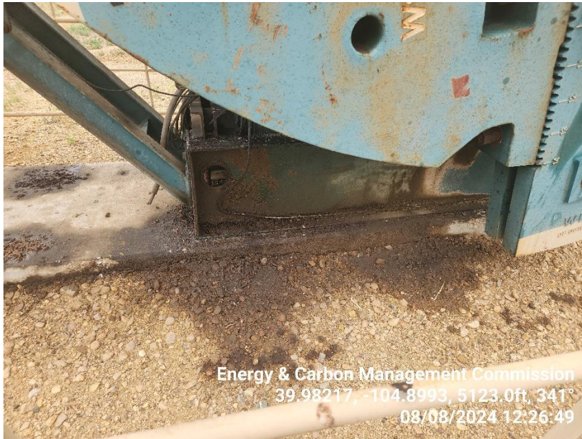
Photo 27 Stained soil on & at the Pump Jack base.
