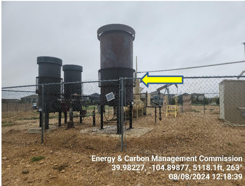
Photo 9 ECDs, The closest has fire damage.
