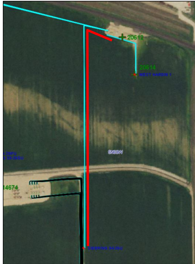
Photo 4. Red line illustrates off-location flowline from the subject well (API 123-25209) to the associated tank battery (to the north). Operator is required to submit a Form 44 Off-Location Flowline Abandonment Notice per Rule 1105.f.(2), therefore, this location will remain "In-Process" until ECMC receives the required notice.
