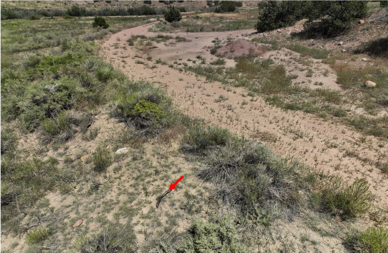
Photo 3. Drone aerial photo facing northeast toward the abandoned wellsite which was never reclaimed. Guyline anchor cable still remains at red arrow. Previous corrective action was not completed.
