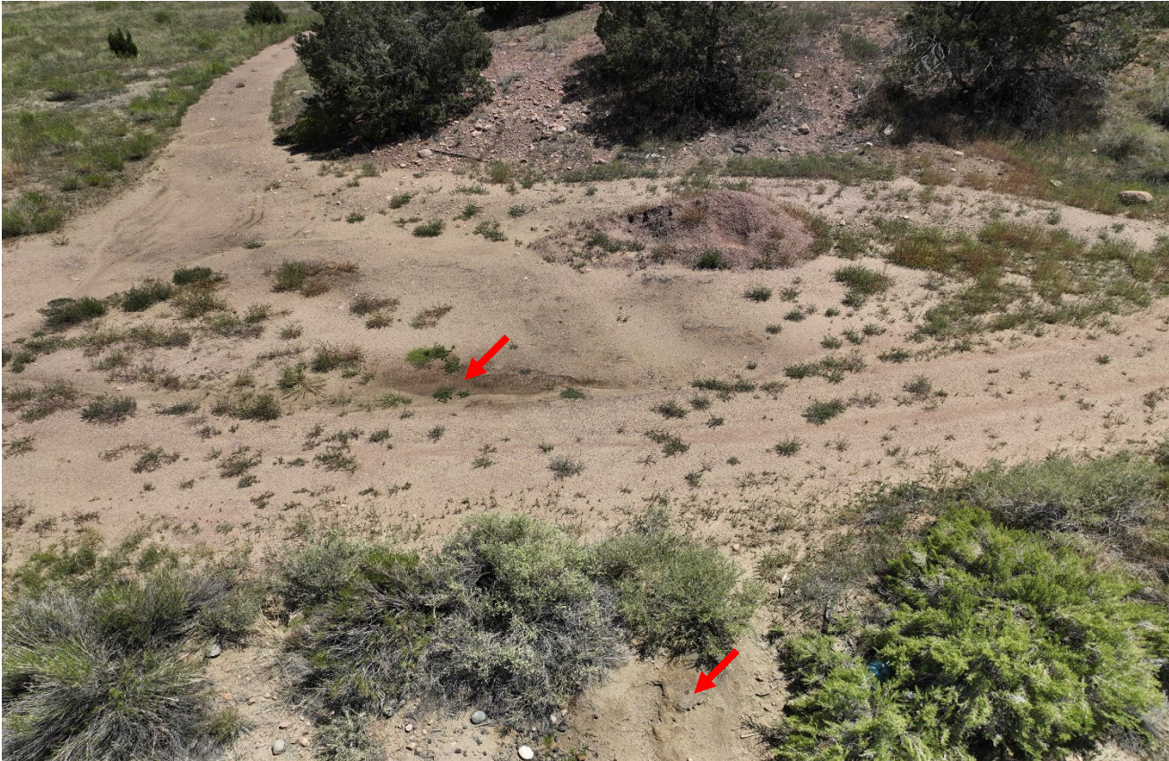
Photo 5. There are oil stained soils in this area at the abandoned well. Impacted soils need to be excavated and removed. Red arrows point to the areas where stained soil is evident.
