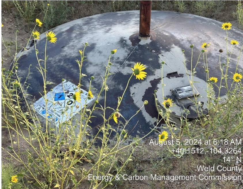
Missing Capacity Label
