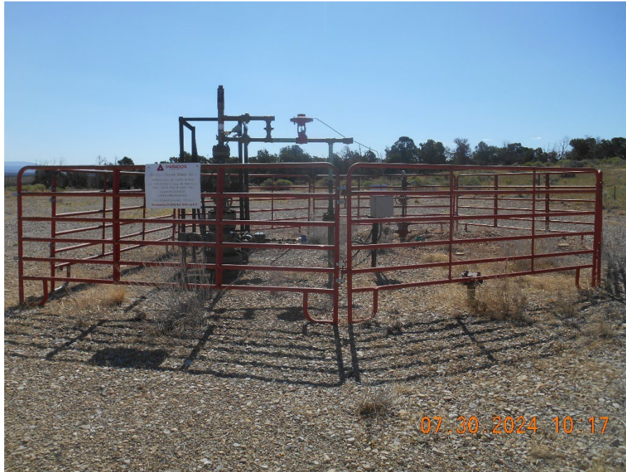
Wellhead with fence and sign
