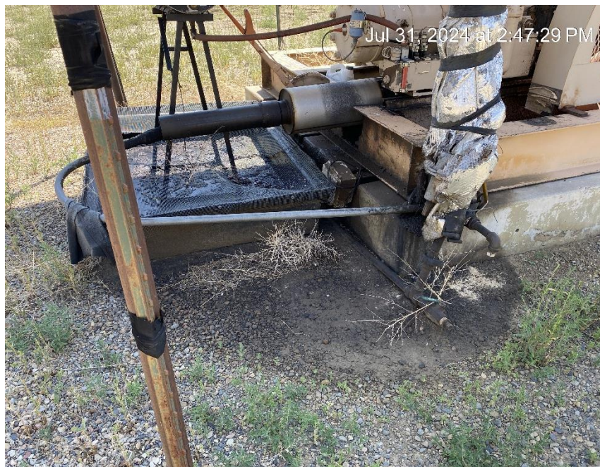
Leaking equipment with oily waste and stained soil
