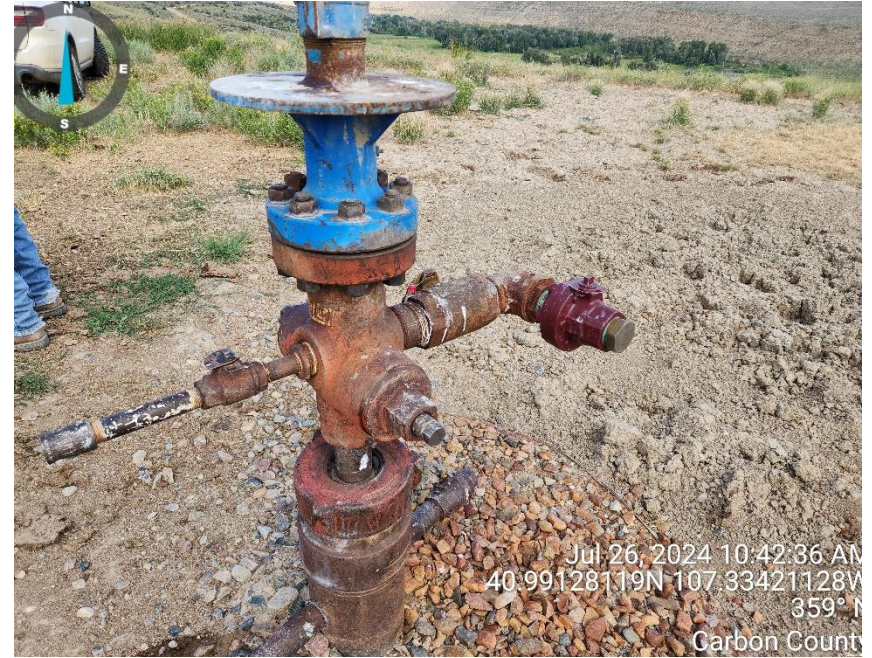
A new 2" valve and plug have been installed since the last field inspection of this location.
