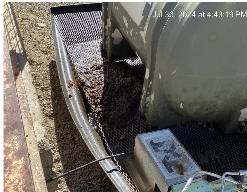
Oily waste on top of containment
