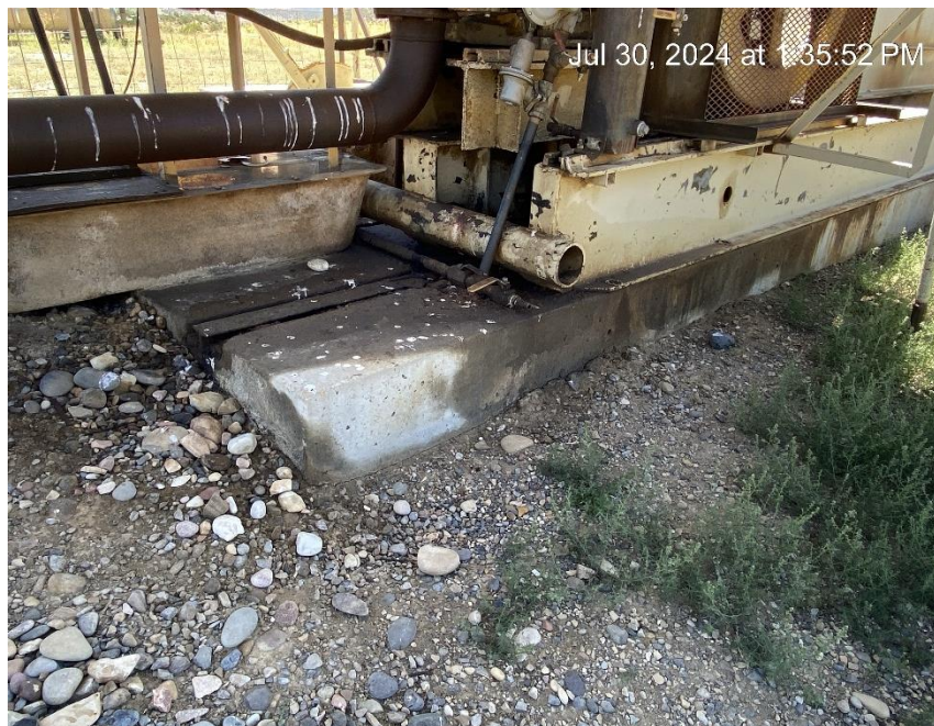
Leaking equipment and stained soil
