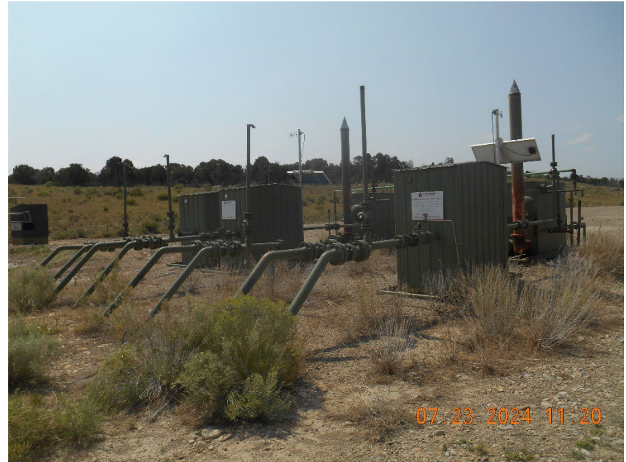
Separators & Meter housings
