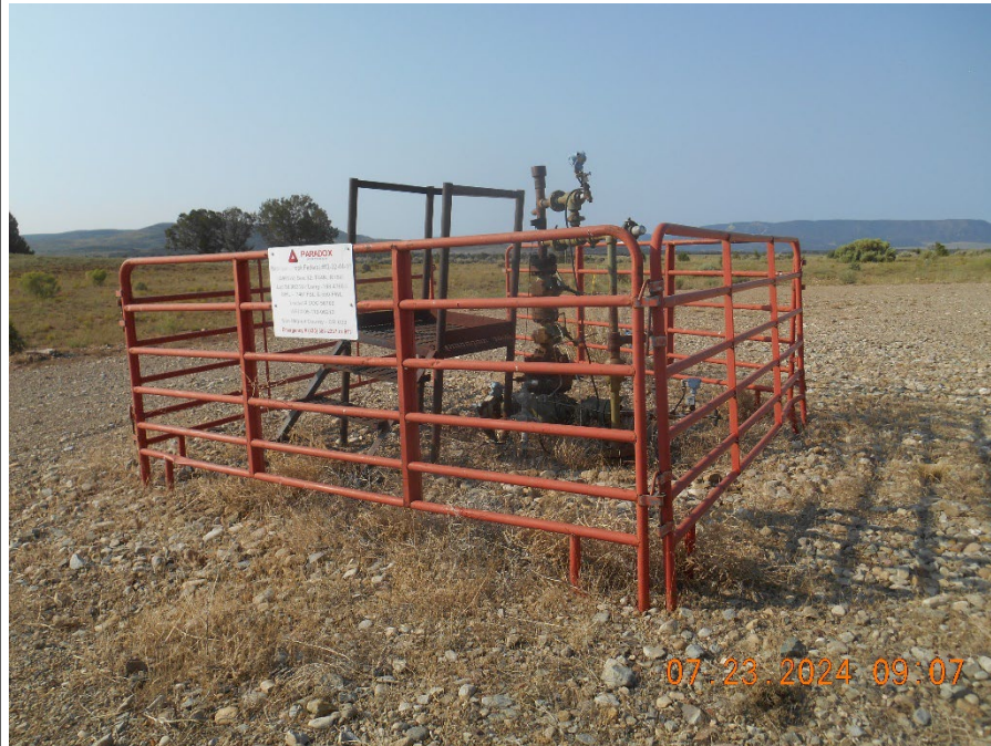
Wellhead with sign and fence. Temporarily abandoned.
