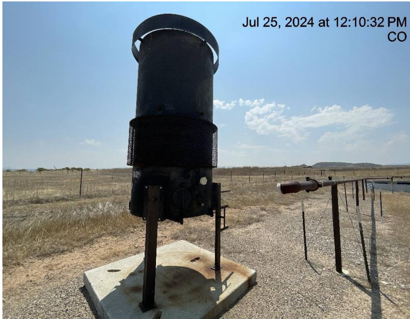
Photo # 3247 Unused equipment/ECD disconnected & not in use
