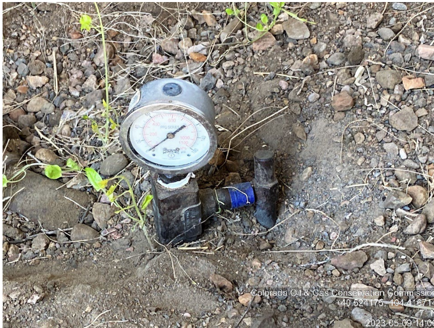
Photo #5 NGL C7A UIC Injection Well Bradenhead Press: 0 psig Active Injection prior photo
