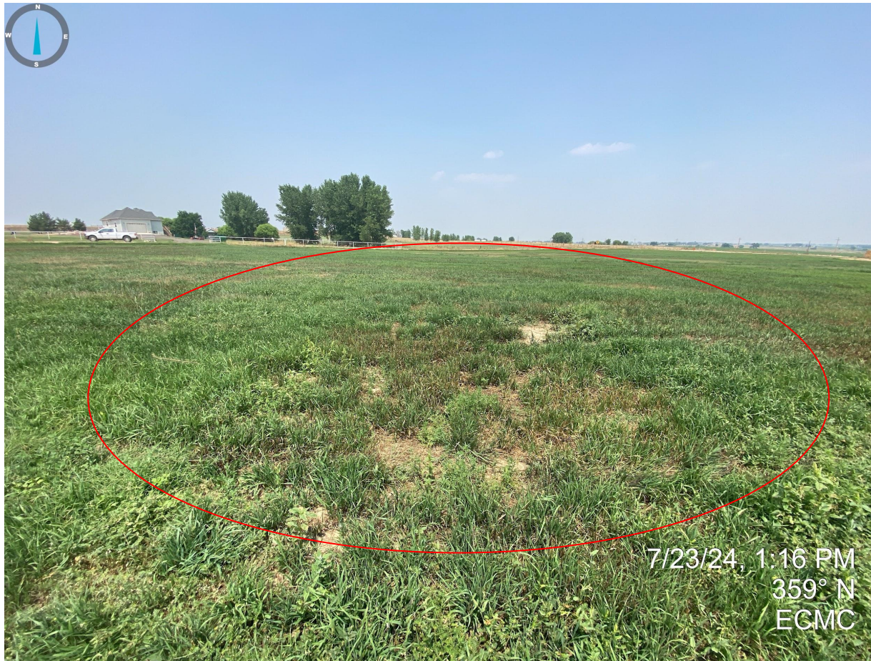
Photo 1. Facing north. The former well location has subsided approximately 1-1.5' bsg. Additional reclamation activities are required to restore grade in order to match the adjacent topography.
