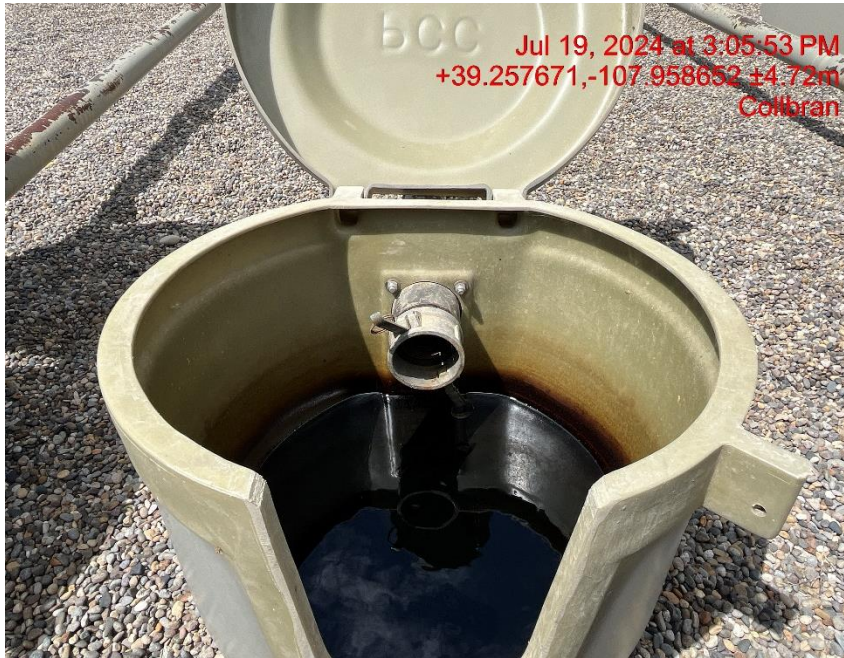
Open ended load line - Photo #03560
