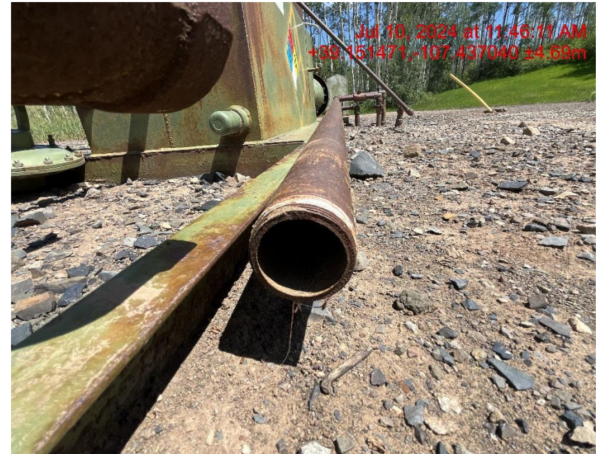
Open ended piping/wildlife hazard - Photo #03486
