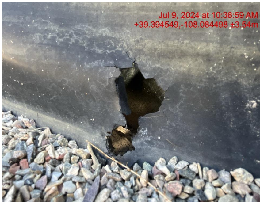
Hole in containment liner - Photo #03406
