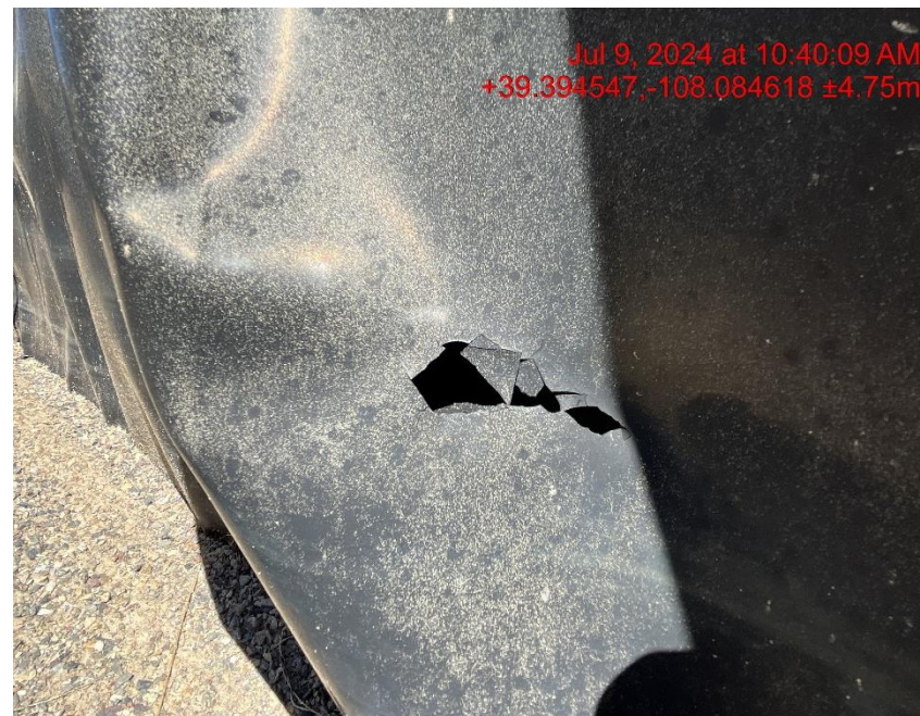
Hole in containment liner - Photo #03408
