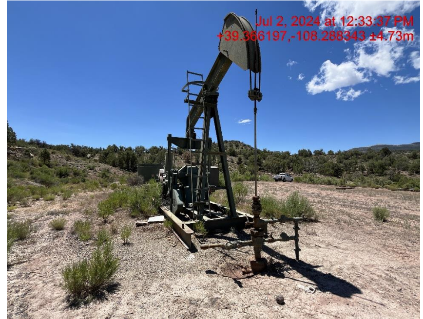
Well head and Pump jack - Photo #03231
